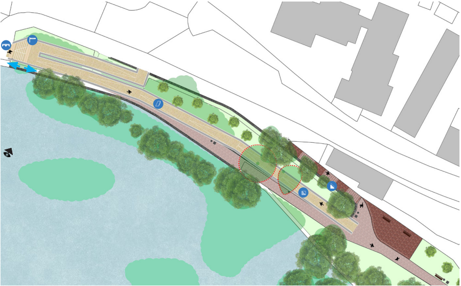
Cynllun opsiwn 1 Grisiau a ramp: strwythur ramp arfaethedig ( gradd 1:20) Step and ramp option 1 plan: Proposed ramp structure at 1:20
