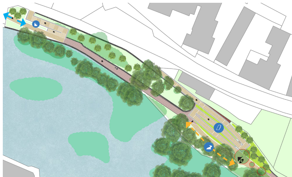
Cynllun opsiwn 2 Grisïau a ramp: strwythur ramparfaethedig ( gradd 1:20) Step and ramp option 2 plan: Proposed ramp structure at 1:20
