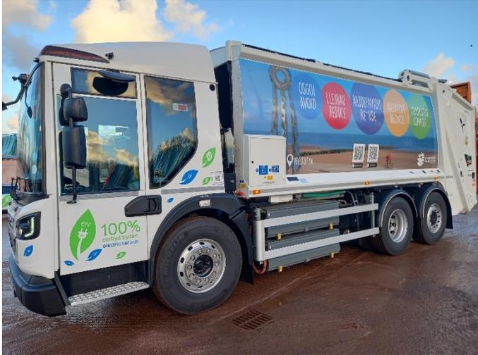
We added two Dennis Eagle e-Collect lorries to the waste collection fleet. Both lorries are used on the county's northern rounds which will include Rhyl, Prestatyn and down to the Trefnant area. They are able to put in up to 100 miles and 1000 bin lifts per single charge.
